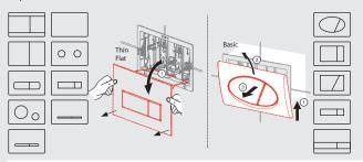
Remove the complete flush plate from the concealed cistern. First of all release the locks used to fasten the flush plate frame. Then use the side clamps to release the flush plate itself and remove it.
