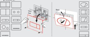
Remove the complete flush plate from the concealed cistern. First of all release the locks used to fasten the flush plate frame. Then use the side clamps to release the flush plate itself and remove it.
