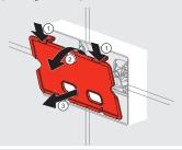
5. Remove the flushing mechanism, which controls the flush valve rod.
