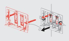
3 Remove the inner plate separating the flush plate from the concealed cistern. You can remove the inner plate by clicking out the grips on the upper edge of the plate.
