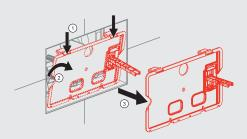
5. Remove the flushing mechanism, which controls the flush valve rod.
