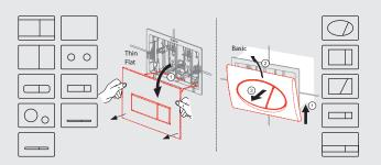
Remove the complete flush plate from the concealed cistern. First of all release the locks used to fasten the flush plate frame. Then use the side clamps to release the flush plate itself and remove it.
