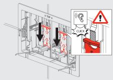
4. Put the flush plate back, check the compression clearance – it should be 1–2 mm.
