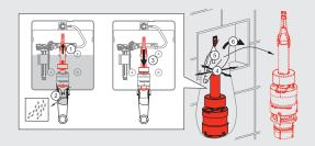
9. Increasing the flushing water volume on the flush valve.
