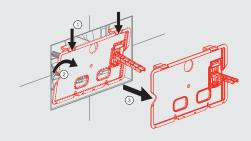
5. Remove the flushing mechanism, which controls the flush valve rod.
