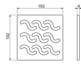
Application For floor drains with a grid size 105×105 mm For use indoors and outdoors
