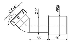
Application For shower wastes and traps For bath wastes and traps in combination with A53-6/4"
