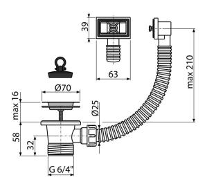
Application For sink with overflow For sink wastes and traps
