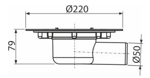
Application For floor drains For use indoors and outdoors
