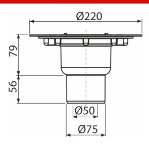
Application For floor drains For use indoors and outdoors
