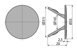
Application For flushing tanks intended for blind plugging the water inlet
