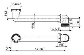
Application For sink wastes and traps To save space under the sink
