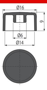
For outdoor drain channels and outdoor drain boxes with composite grids To cover the screws for fixing the composite grid
