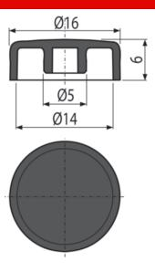
For outdoor drain channels and outdoor drain boxes with cast iron grids To cover the screws for fixing the cast iron grid
