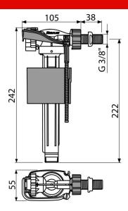
Application For installation on the side of the cistern
