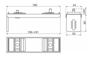
Application For ALCASYSTEM construction For anchoring the ALCASYSTEM construction to the wall
