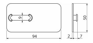
Application For ALCASYSTEM construction For sound insulation of profile holders (AS-P012, AS-P011, AS-P013, AS-P014)
