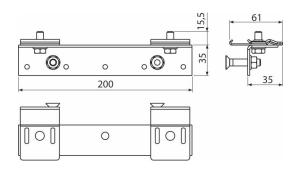
Application For ALCASYSTEM construction For mounting wooden timbering – thickness 25 mm
